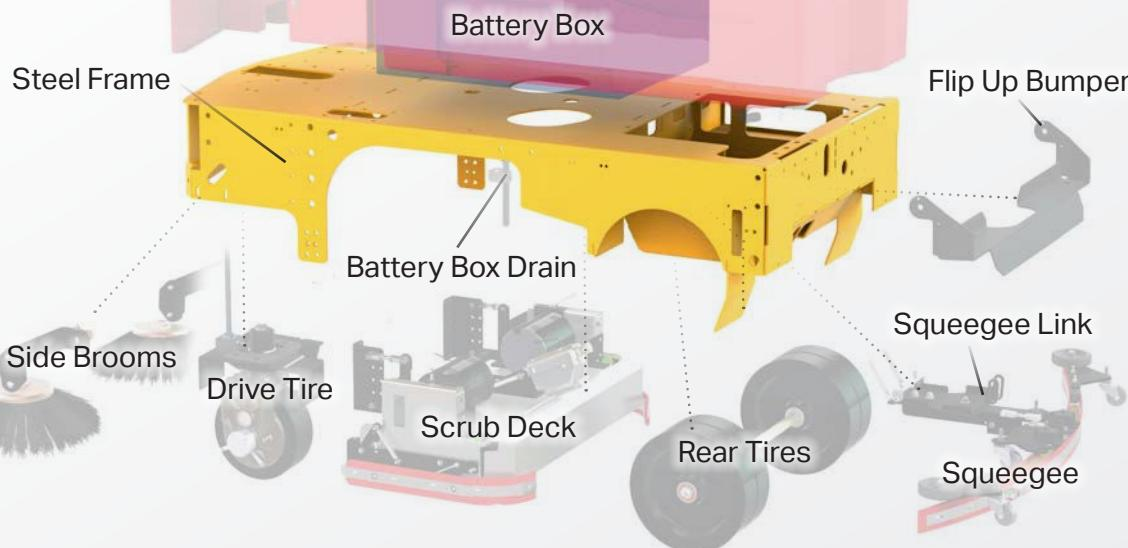
We spend the extra time and money to through-bolt with stainless fasteners for longevity and service ease in the future. Some of our larger rider scrubbers have 750-lbs in batteries in a full height poly liner, supported by the steel frame.
